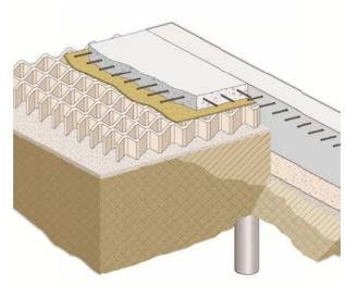
Where swelling or shrinking soils are known to be present, National Building Code of Canada (NBC) provisions require that soil movement be provided for in the design of structures likely to be damaged. **GeoSpan** and **GeoVoid** compressible fill material properties assist designers in addressing the NBC requirements as follows:
