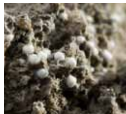
Elemix additive (white polymeric spheres) distributes uniformly in concrete to reduce weight
