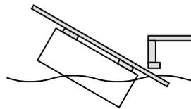
3. Tilt crib; push under wharf using the cross members as handles.
