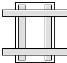
2. Build a crib of 2" x 8" (38 mm x 190 mm) lumber and fasten it to the PlastiSpan billets. Cross members should be longer than width of wharf.
