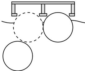
1. Puncture existing drums and allow them to sink for removal; remove two at a time.
