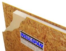
Insulspan SIPs provide continuous expanded polystyrene (EPS) insulation with minimal dimensional lumber studs that create a thermal “bridge” of heat transfer to the exterior. Building with large panels also means better air tightness for even greater energy efficiency, comfort, and indoor air quality.
