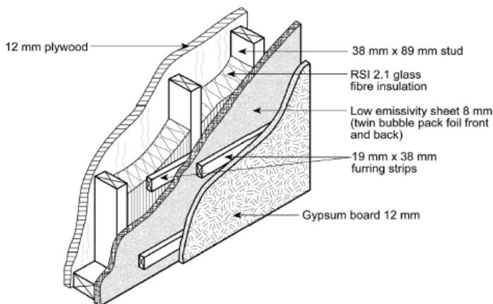
**Figure 1 - CCMC Evaluated Wall Assembly**
