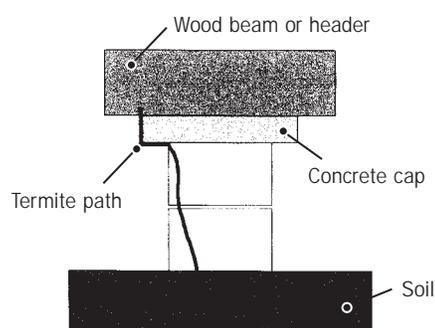
Brick and hollow block piers can be made more termite resistant through the use of solid concrete caps. Caps force termites tunneling within the hollow blocks to move to the exterior of the cap where they can be detected.
