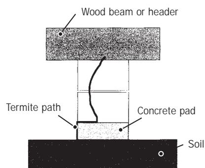
Solid concrete pads also force termites to build exterior mud tubes for easy detection. Pads are easiest to treat since only the soil around the perimeter needs treatment, not the interior of the pier. The pad should have no cracks and extend above the soil.
