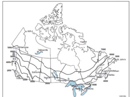
NECB 2011, Appendix Figure A-1.1.4.1.(1) – Contour Map of Approximate Annual Heating Degree Days
