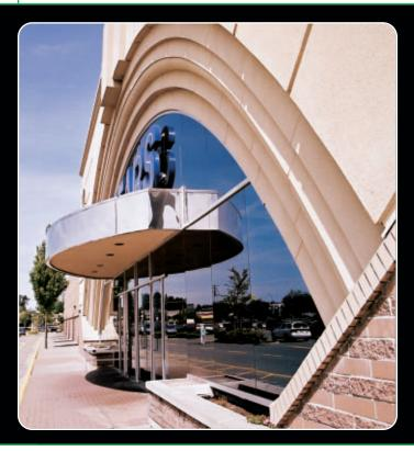
PlastiSpan insulation is used as the insulation component in exterior finish systems. Exterior Insulation Finish Systems (EIFS) are popular external cladding systems, which are applied over PlastiSpan insulation to provide durable surfaces.
