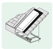
Ideal where exposed timber deck is chosen inside building finish and slope is sufficient to allow the use of shingles, shakes or tiles.
