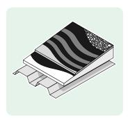
Provides the positive slope to drain while maintaining the structural and economic advantages of a flat roof deck system.
