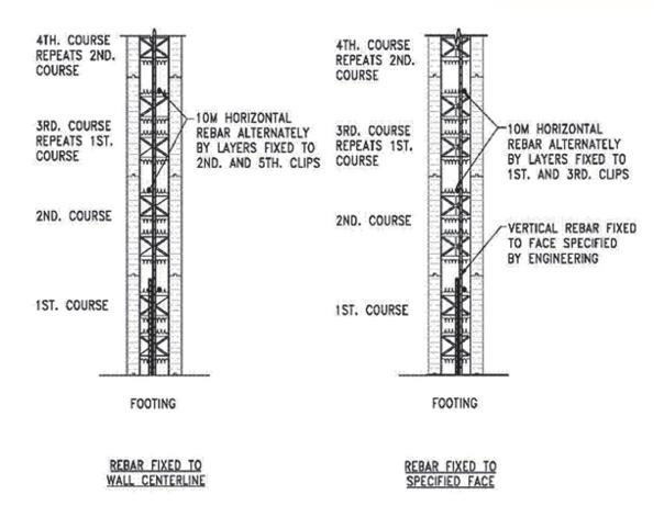
Note: Horizontal & vertical rebar overlapped 450 mm (18") for 10M bar and 650 mm (26") for 15M bars
