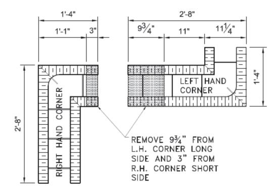
Figure 26: Two-Foot Corners – 152 mm (6") Block.
