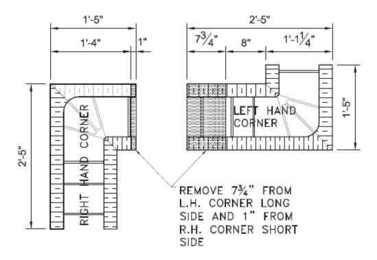
Figure 27: Two-Foot Corners – 203 mm (8") Block.
