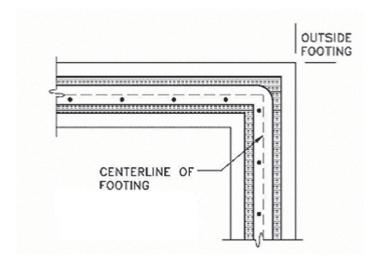
Figure 2: Placement of Block on Concrete Footings
