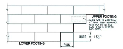
Figure 3: Diagram to illustrate step footings.
