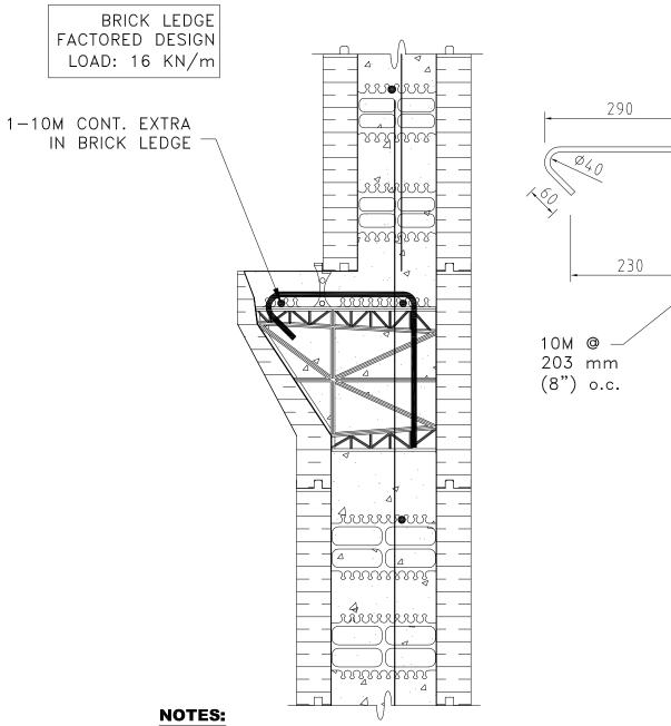
1. DETAIL TO BE USED IN CONJUNCTION WITH ADVANTAGE ICF SYSTEM TECHNICAL & INSTALLATION MANUAL.
